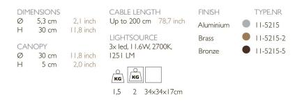
STANDARD The fixture is supplied with lamps. Black canopy with cover plate in matching colour of the fixture. Leading and trailing edge dimmable. Nickel, natural brass or blackened natural brass.
